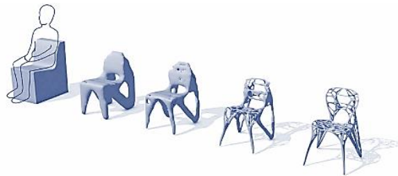
Fig. 1 The formal alternatives for designing a chair according to the performance parameters [24].
