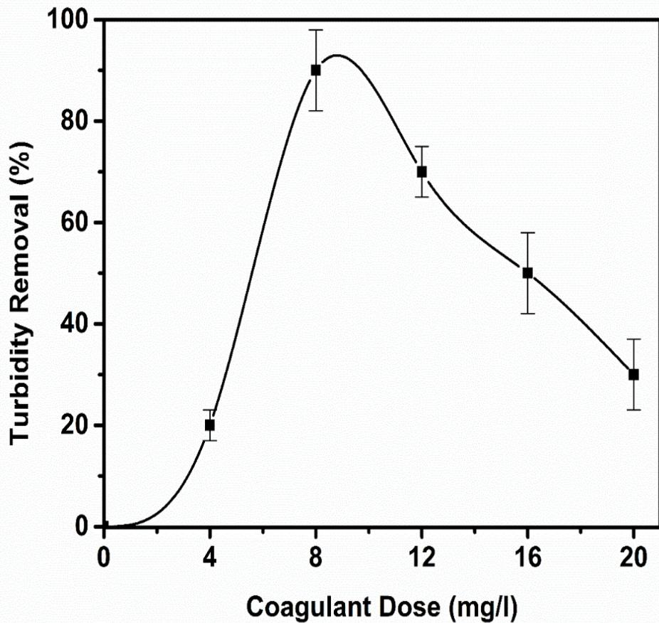
Fig. 2. Effect of coagulant (Aleo-vera) dose on turbidity removal.
