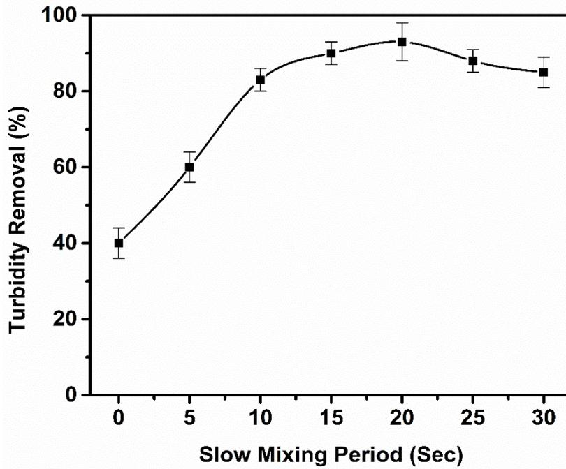
Fig. 6. Effect of slow mixing period on turbidity removal.
