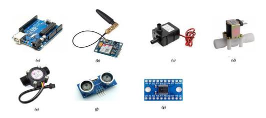
Fig. 5 Prototype components and their respective models (a) Arduino Uno R3 Microcontroller, (b) SIM800L V2 5V Wireless GSM GPRS Module, (c) AD20P-1230C Ultra-Quiet DC 12V 3M 240L/H Brushless Submersible Water Pump, (d) 12V Electric Solenoid Valve 90 Magnetic N/C Water Air Inlet Flow Switch, (e) YF-S201 Water Flow Measurement Sensor with 1-30 Liter/min Flow Rate, (f) HC-SR04 Ultrasonic Sensor, (g) 3.3V to 5V 4 Channels IIC I2C Logic Level Converter Bi-Directional Shifter Module.
