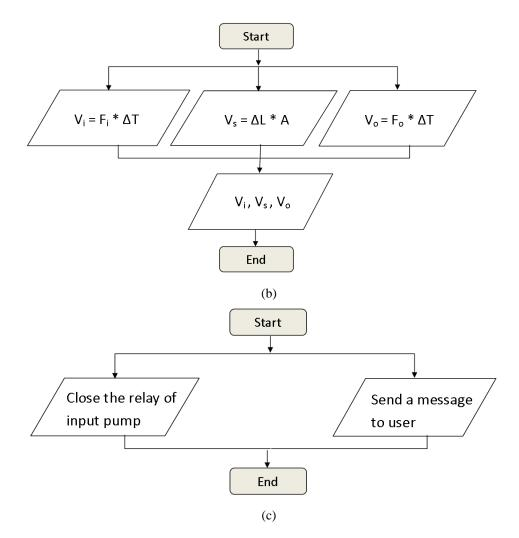
Fig. 4 (a) System Flowchart, (b) Normal Mode Flowchart, and (c) Outage and Leakage Modes Flowchart.
