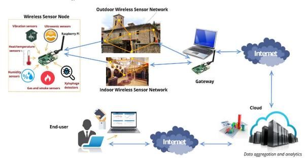
Fig. 12. The general structure of the proposed monitoring system based on (IoT) in the church building[32].
