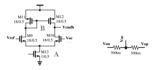
Fig. 3. The schematic diagram of the CMFB.
