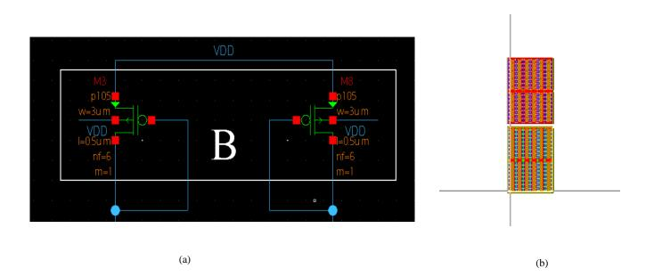
Fig. 6. CMFB subblock B, (a) The schematic, (b) The automated layout.
