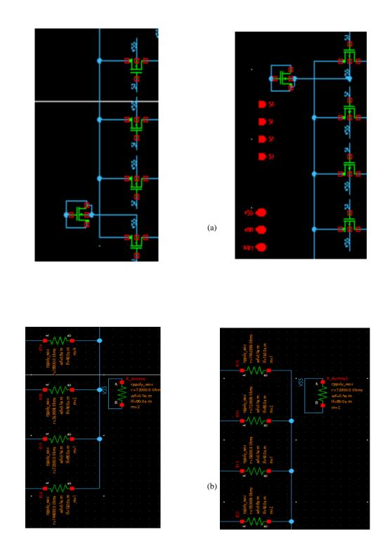
Fig. 9. Schematic of the top-level VGA two subblocks, (a) VGA transistors, (b) VGA resistors.
