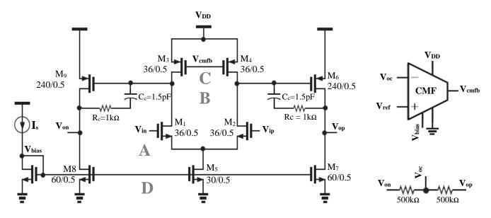
Fig. 4. The schematic diagram of the OTA.
