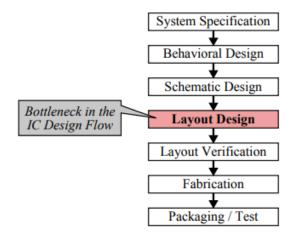
Fig. 1. Simplified illustration of the integrated circuit design flow.
