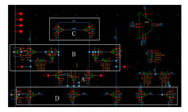
Fig. 7. Schematic of OTA subblocks.
