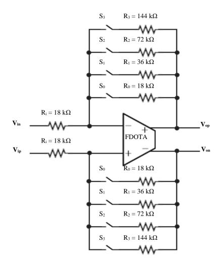
Fig. 2. The schematic diagram of the top level of the VGA.
