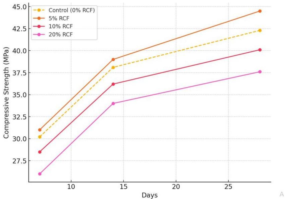
Figure 1: Compressive Strength of Slag-RCF Concrete at 7, 14, and 28 Days.
