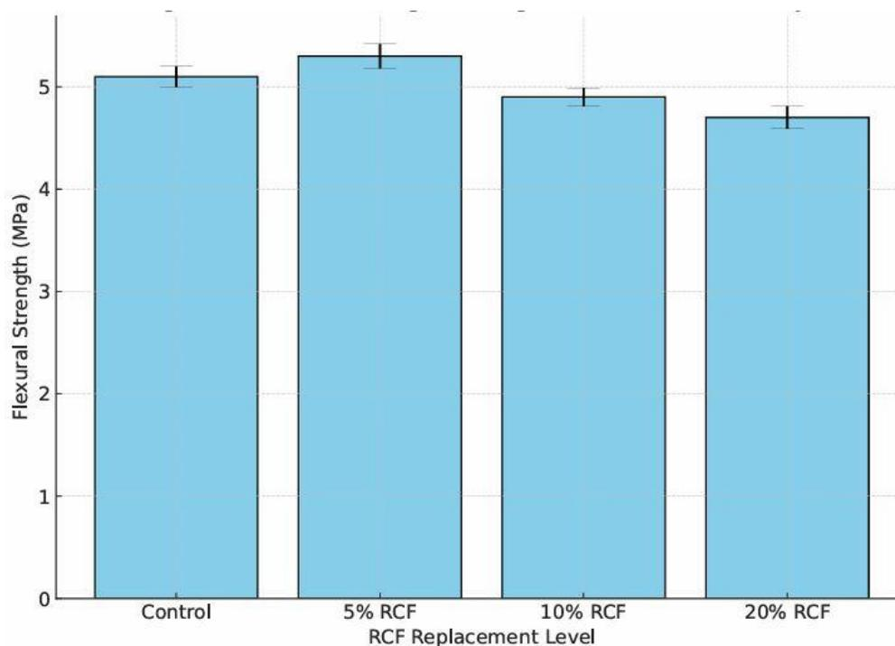
Figure 2: Flexural Strength of Slag-RCF Concrete at 28 Days.
